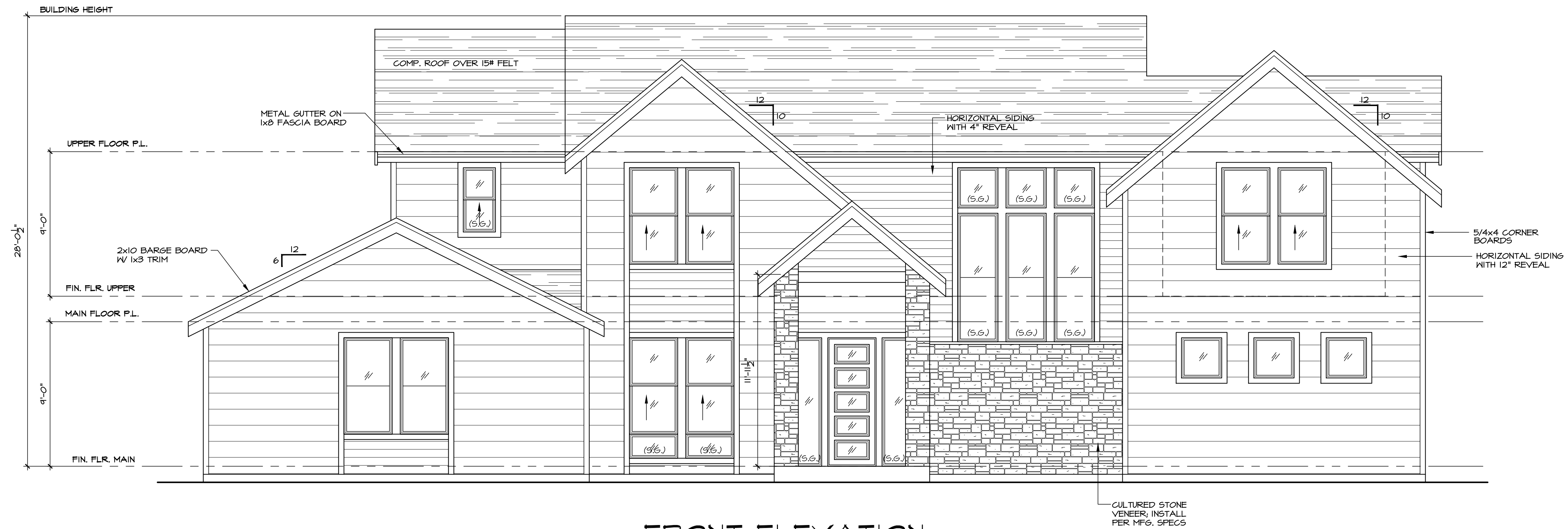
FRONT ELEVATION SEE GENERAL NOTES SCALE: 1/4" = 1'-0"
