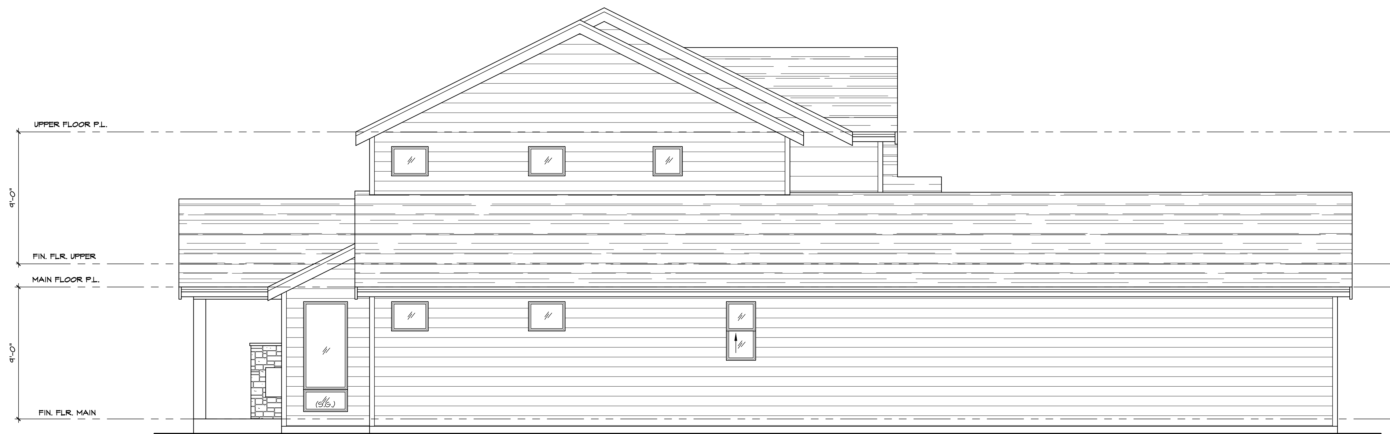
LEFT ELEVATION SEE GENERAL NOTES SCALE: 1/4" = 1'-0"
